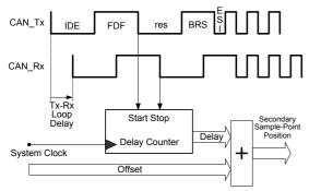
Figure 4: Loop Delay Measurement
