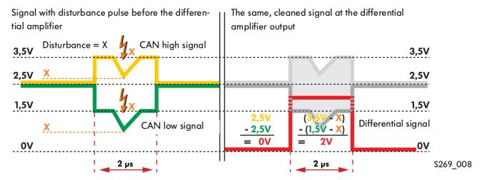
Evaluation of the signals from CAN high and CAN low in the differential amplifier, otherwise known as differential transfer technology, means that the effects of disturbances are practically eliminated. Another advantage of differential transfer technology is the fact that fluctuations in the onboard supply (e.g. when the engine is started) do not affect the transfer of data to individual control units (transfer security).
