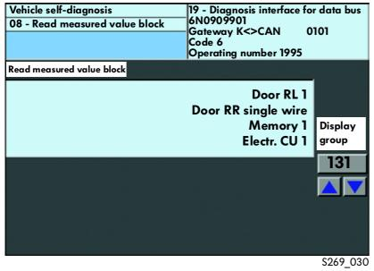
In this case, the "Rear right door control unit" will switch to single wire operation (message; "door RR single wire"), while the other three control units are in dual wire mode (message: "... 1").
