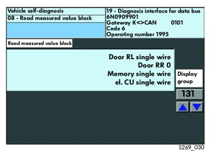
VAS 5051 will report that all control units are in single wire mode and that the "Rear right door control unit" has no communication (message: "door RR 0"). Therefore, a connection to the "rear right control unit" in the CAN low wire is affected by the open circuit.
