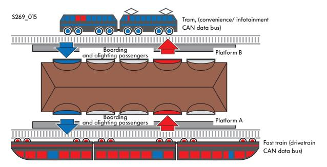
At platform A (otherwise known as the Gateway) of the railway, a fast train arrives (drivetrain CAN data bus, 500 kBit/s) with several hundred passengers onboard.
