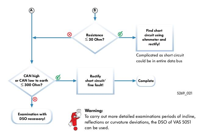
On measurements described as follows, for which the DSO of VAS 5051 is used, the trigger threshold must always be adjusted in addition to the period (horizontal) and voltage sensitivity (vertical). The trigger threshold is the adjustable test voltage on VAS 5051. Recording will start if it is above or below the signal to be measured.
